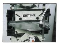
SIMPLEST AUTO FEED System can be used. NO MOVING PARTS! Just the springs and worktable! 20,000 SPRINGS per hour can be ground to better than 2 degrees of squareness.
